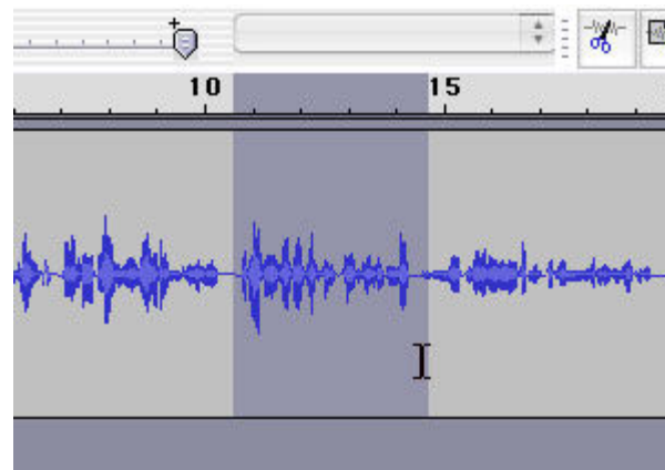
Figure 2. Click and drag over unwanted audio to select it and press the Delete key.
